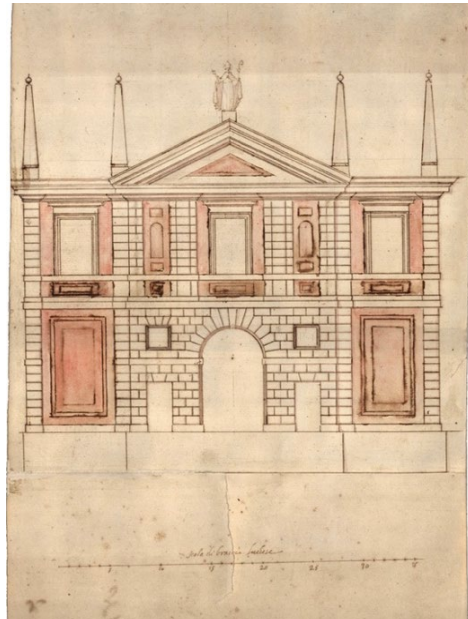
Fig. 5- Muzio Oddi, project for the San Donato gate in Lucca (State Archives of Lucca, Fortifications of the City and State , 42, n. 54).
