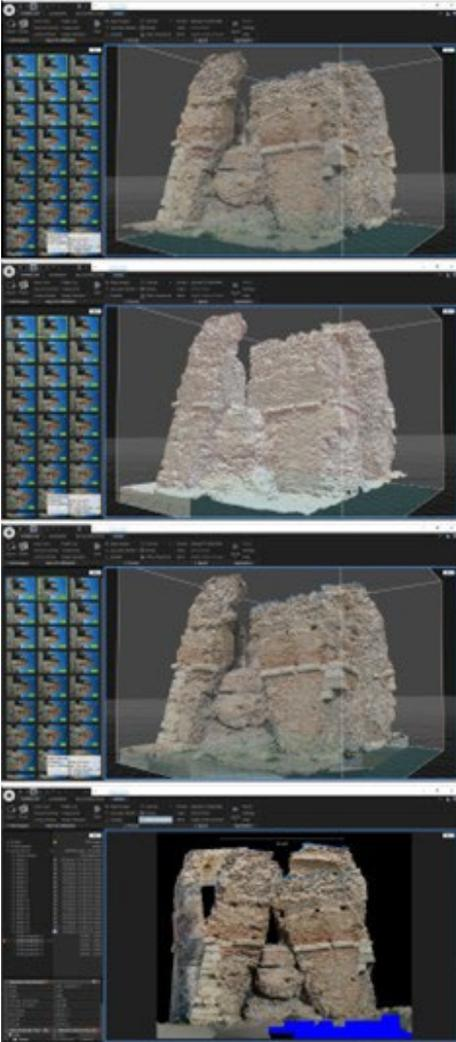
Fig. 6- Photogrammetric processing in EG Reality Capture (graphic elaboration by the authors, 2024).
