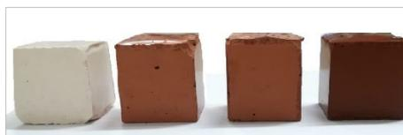
Fig. 2 - Geopolymer samples with different RM amount.
