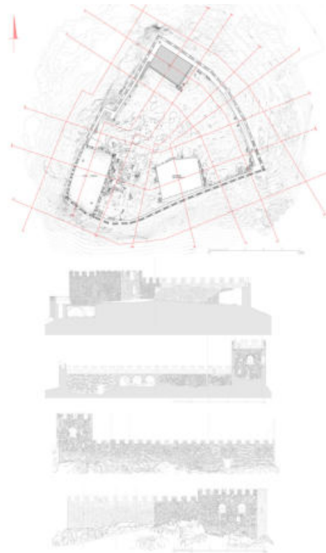
Fig. 3- General drawings of Construction phase 1 of the castle (graphic reconstruction) (Michael Miaoulis & Philippos Kanatouris, 2018)
